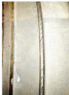
Tread Groove Cracking Figure 311
