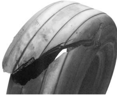
Burst (Tyre Failure) Figure 308
