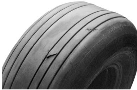
Cut Damage Figure 303
